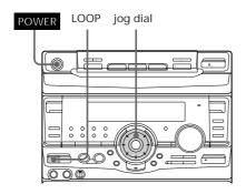
/ Press and hold LOOP during playback at the point you want to start the Loop function, and release to resume normal play.
